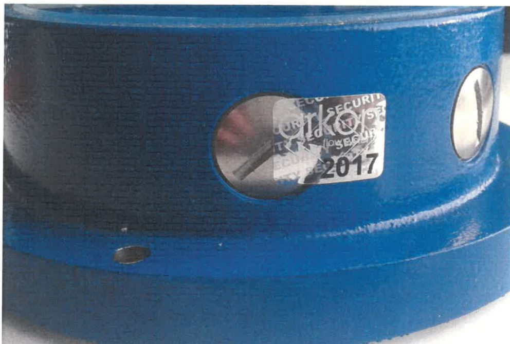
Figure 2: The water meter type MAGB1 – sealing of the screw covering the USB:
