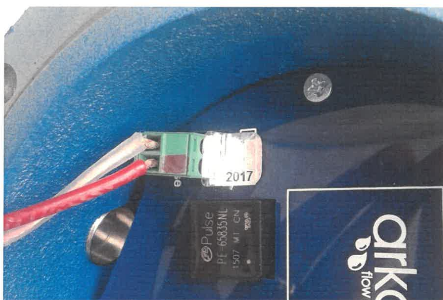
Figure 6: The water meter type MAGB1 – frequency output and RS 485 sealing:
