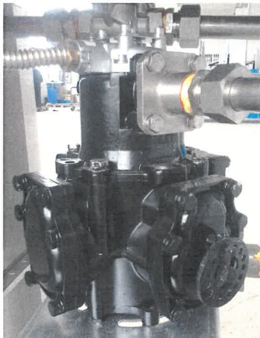
Picture No. 1: NSF1 measurement transducer
