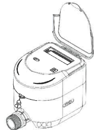
Fig. 3: The sealing of water meter types LXC-15, LXC-20 and LXC-25
