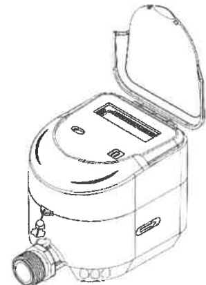
Fig. 3: The sealing of water meter types LXC-15, LXC-20 and LXC-25
