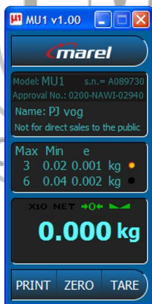
Example of stand alone MU1 PC user interface on a Windows computer
