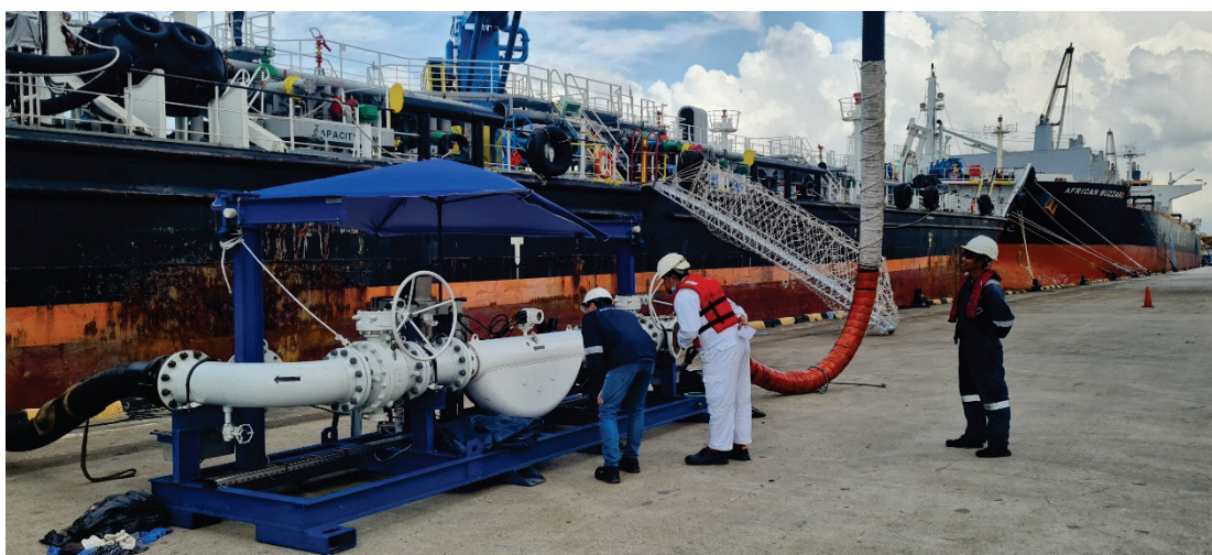
Picture 1: Bunkering operations in process using master meter
