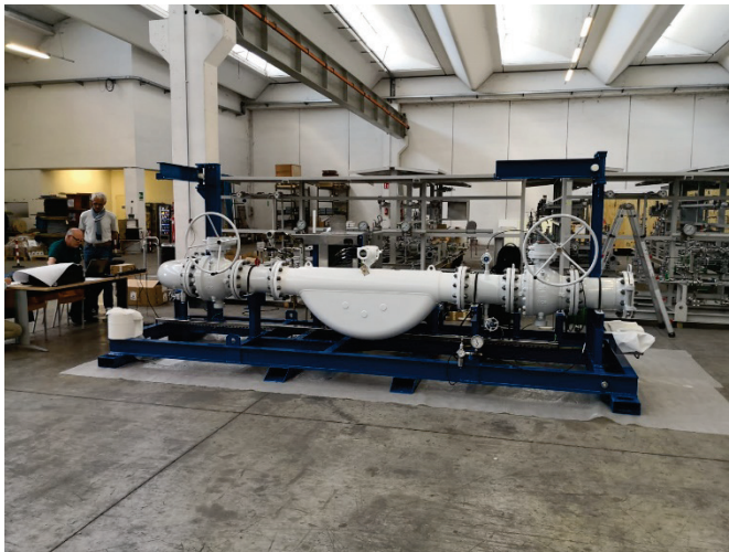
Picture 2: The Master Meter is calibrated annually at Endress+Hauser's flow lab with direct traceability through its highly precision calibration rig in Reinach, Switzerland
