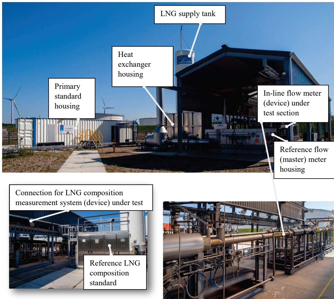
Figure 2: VSL's calibration and test facility for LNG quantity and LNG composition measurement systems, which is fully traceable to the SI units of measurement. Outline of several main components (top, reprocessed from [21]), LNG composition measurement system (device) under test connection point (lower left, reprocessed from [25]), zoom-in of in-line flow meter test section (lower right, reprocessed from [27]).
